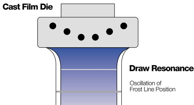
ratio. In general, if the die gap opening is decreased, a previously unstable web will move closer to or into a stable operating region.
